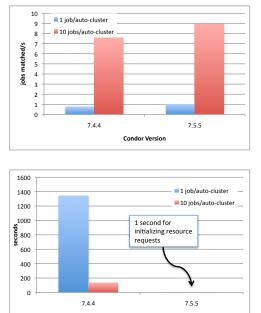
Figure 3. Average number of jobs matched per second while matching 1000 jobs to a pool of 10,000 slots. Higher rates are possible when jobs can be grouped into equivalent sets (autoclusters).
