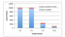
Figure 1. Fsync operations performed by Condor to run a sample workflow: 100 vanilla universe jobs were submitted in clusters of 10; they ran for 20 minutes, were evicted, restarted and ran to completion after an hour. Each job cluster had its own event log. To illustrate fsync optimizations that have been made in response to real-life HEP usage, the jobs each set match\_list\_length=5 and have five attributes with \$\$() references.
